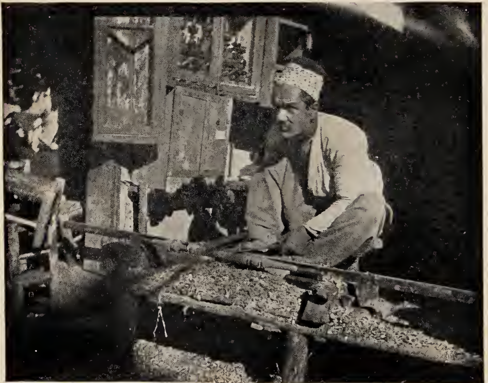
A wood-turner of Damascus. He watches the ever-passing throng, turning the stick with a bow and a loose string, and holding the chisel with his toes
